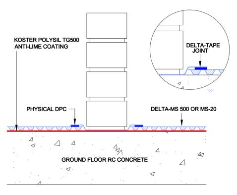
A CONTINUATION OF THE FLOOR MEMBRANE CAN BE ACHIEVED BY EXTENDING THE PHYSICAL DPC. BEYOND THE NEW WALL TO OVERLAP ONTO SYSTEM 500. THIS IS THEN SEALED WITH DELTA-TAPE.
