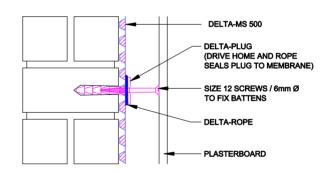
PRE-TREATED BATTENS CAN BE FIXED INTO DELTA-PLUGS USING SIZE 12 SCREWS.
