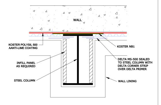
STEEL BEAM DETAIL (lapped DPC joint)
