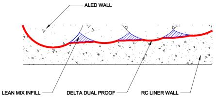
\* THE UNDERSLAB DELTA DUAL PROOF SHOULD TERMINATE AT LEAST 150mm ABOVE THE TOP OF THE POURED SLAB
