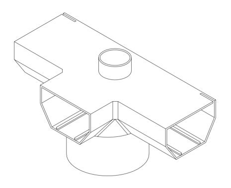
THE T-PIECE DESIGN ALLOWS FOR 3 CHANNEL RUNS TO BE CONNECTED IF REQUIRED TO THE SINGLE OUTLET FOR CONVENIENCE - ENABLING PERIMETER AND CROSS FLOOR DRAINAGE CHANNELS TO BE EASILY DISCHARGED INTO THE SUMP AND PUMP SYSTEM
