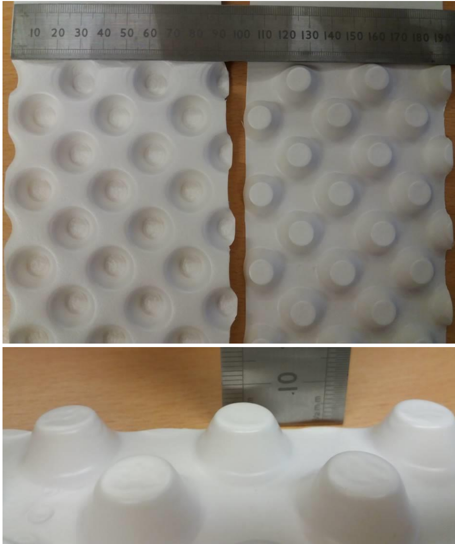
Figure A.1: EN ISO 11925-2 test sample, as received
