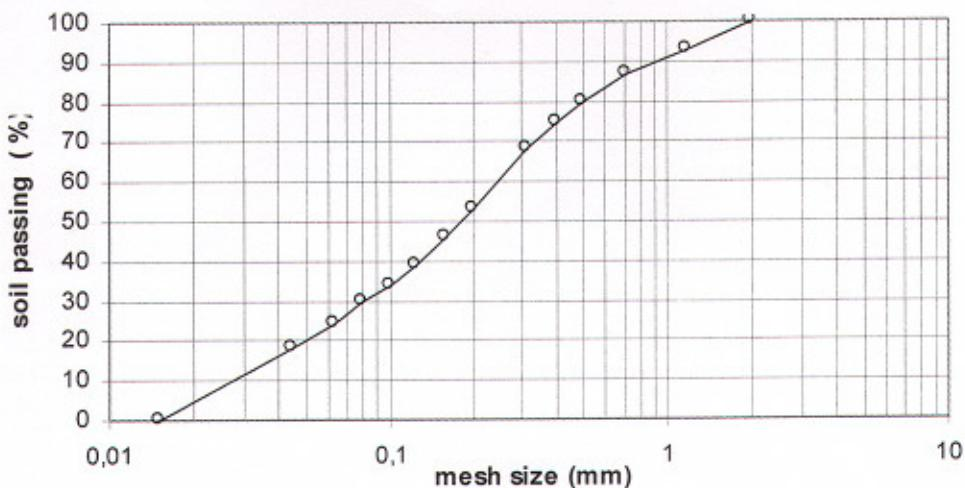
cumulative particle size distribution curve of the soil passing
